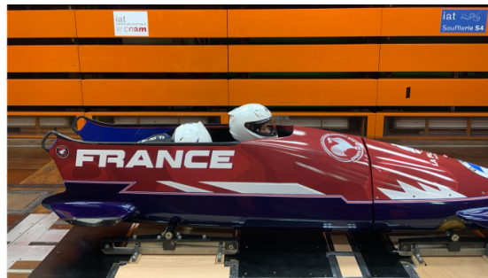
Experimental set-up used to measure the aerodynamic coefficient SC_z of a two-person bobsleigh
